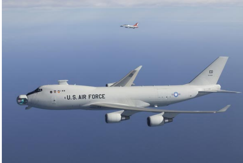
Figure 1.1: Airborne Laser. The COIL integrated into the Boeing 747 provides the needed firepower to destroy enemy missiles in the boost phase. The ABL is designed to operate at high-altitudes over a designated battlefield near missile launch areas. The turret at the front of the aircraft accurately focuses the laser beam and provides the needed atmospheric compensation. Courtesy of Boeing Corporation, photo credit: USAF Photo by Jim Shryne. http://www.boeing.com/defense-space/military/abl/
